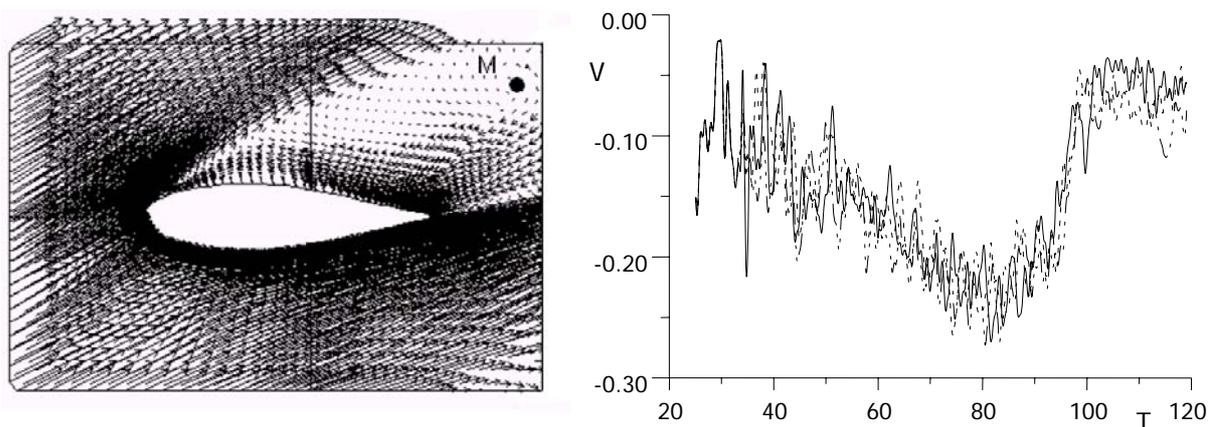
Figure 5. Snapshot of separated flow past a NACA-airfoil strut and velocity oscillations at compatible monitoring points, M, placed in neighboring sectors of the diffuser.
