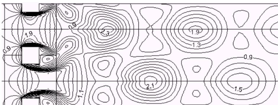
Figure 7. Snapshot of velocity isolines in the two-pitch domain 2D URANS solution.
