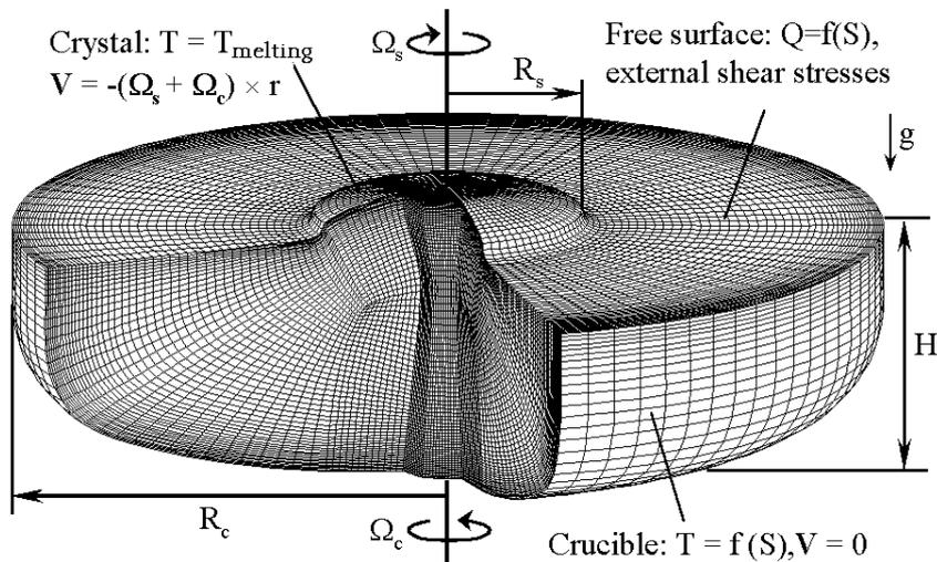
Figure 2. Block-structured computational grid and boundary conditions for direct numerical simulation of turbulent silicon melt convection in a Czochralski crystal growth process.
