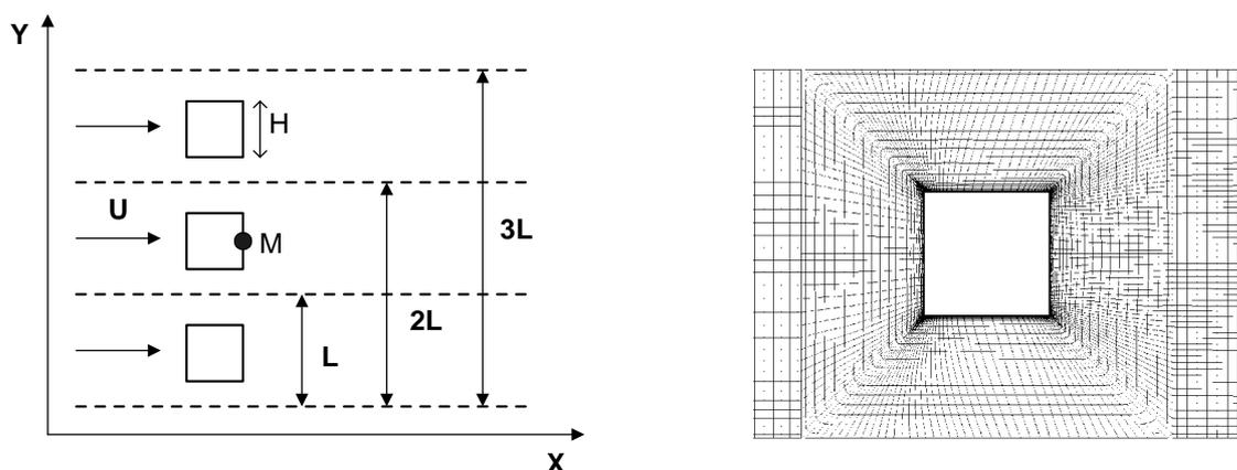
Figure 6. Scheme of flow through a square-bar row and a fragment of an H-O-H grid.
