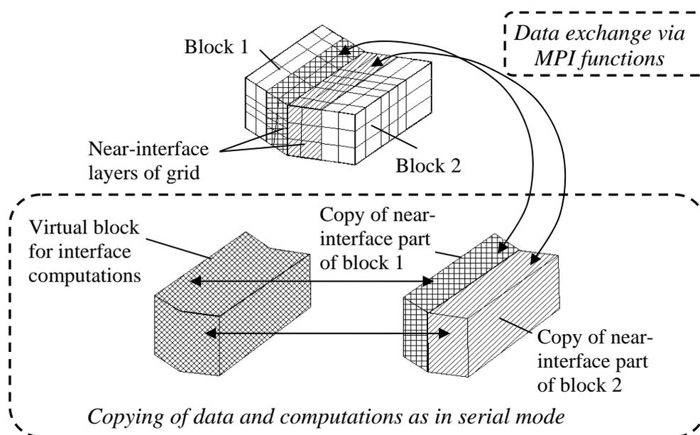
Figure 1. Scheme of data exchange in the parallel version of the code SINF.
