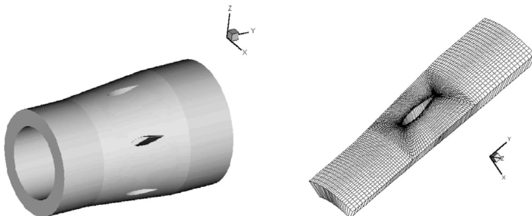
Figure 4. “Solid-gas” model of a gas turbine exhaust diffuser and an H-O-H computational grid for a 60-deg sector of the diffuser.
