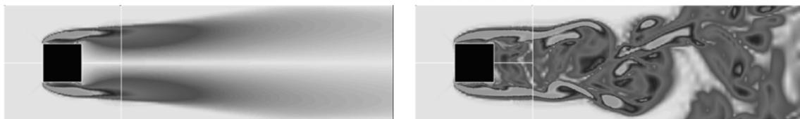
Figure 8. Steady-state vorticity field in the 2D RANS solution (left) and a snapshot of unsteady vorticity field in the 3D DES solution (right) for the one-pitch domain.
