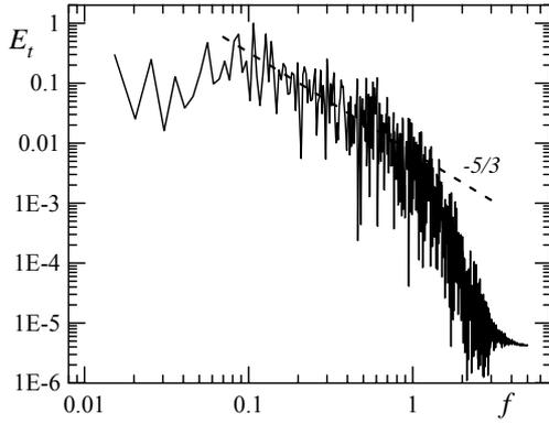
Fig. 6. Power spectral density of temperature fluctuations ( $z = 0.25, r = 0$ ). Mercury,  $Ra = 5 \times 10^8$ .
