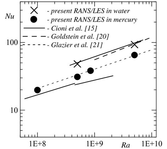
Fig. 7. Nusselt vs Rayleigh numbers in comparison with experimental data.
