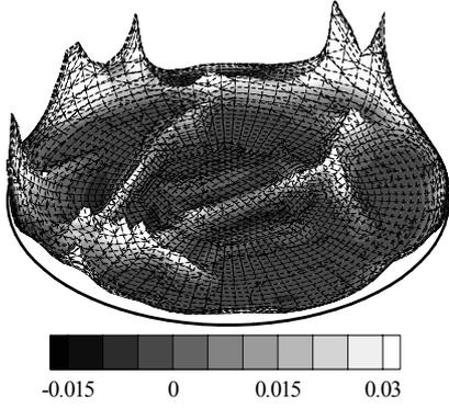
Fig. 3. Temperature isosurface  $\Theta = 0.9$  colored by vertical velocity. Mercury,  $Ra = 5 \times 10^8$ .
