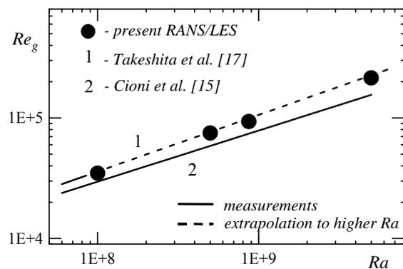
Fig. 2. Reynolds vs Rayleigh numbers for mercury in comparison with experimental data.
