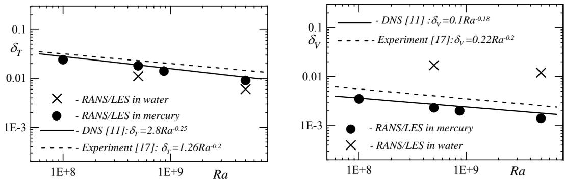
Fig. 5. Thermal (left) and viscous (right) boundary layer thicknesses as functions of the Rayleigh number. Comparison with extrapolations of experimental and DNS data for mercury to higher  $Ra$ .
