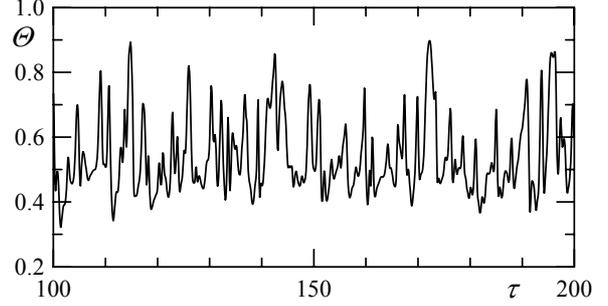
Fig. 4. Temperature fluctuations near the bottom plate ( $z = 0.03$ ,  $r = 0$ ). Mercury,  $Ra = 5 \times 10^8$ .
